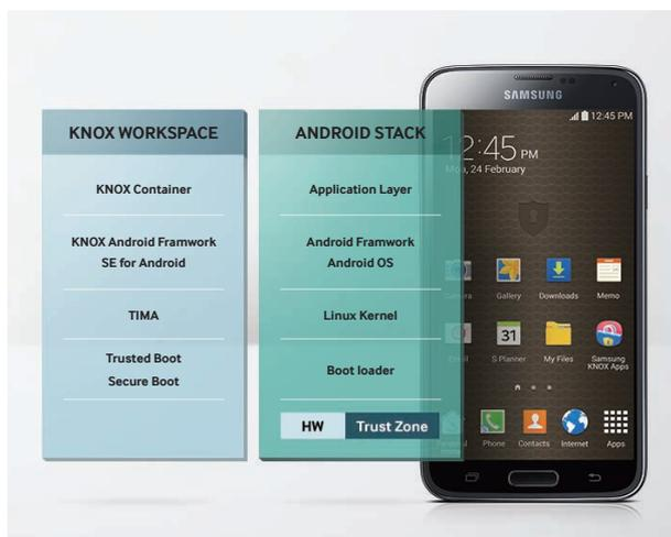
Figure 1. KNOX enhanced platform layers
